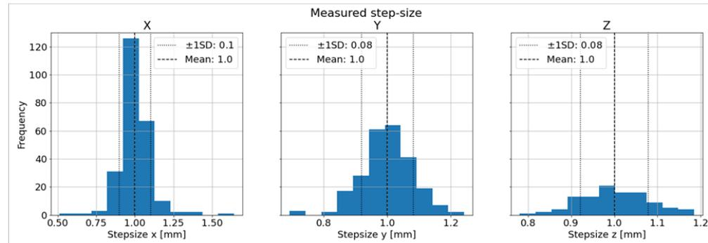
Fig. 4: Combined deviation of filmed position from position recorded by phantom for each axis on fig. 2.
