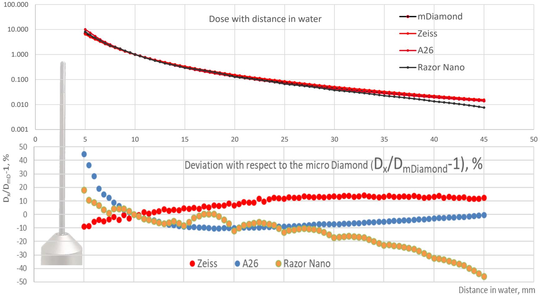
**Measurements vs Zeiss provided user data. INTRABEAM 40 mm spherical app.**
