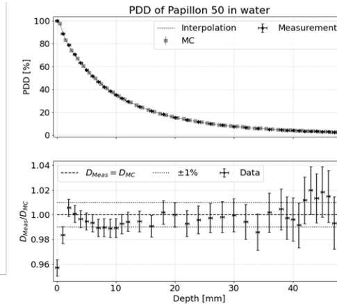
Fig. 5: PDD as measured with PSD and scored with MC.
