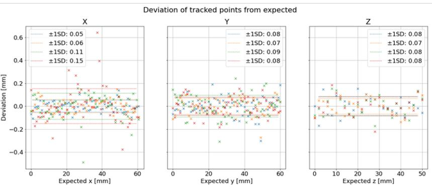
Fig. 3: Deviation of filmed position from position recorded by phantom for the individual tracked points on fig. 2.
