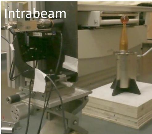
X-Ray spectrometry of the beam emitted by the eBT system
